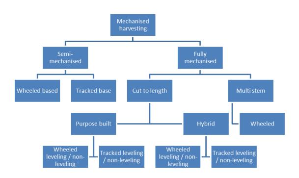
Figure 7: Classification of mechanised harvesting systems
