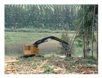
Photo 11a: Tracked single stem harvester (CTL system)
