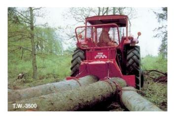
Photo 2a: Tractor with winch (www.logloader.com)
