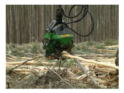
Photo 9: Locally designed debarking head<sup>3</sup>
