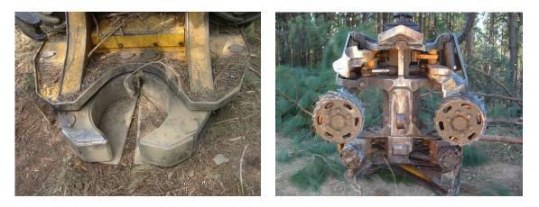
Photo 13 (left): Shear type felling head<sup>7</sup>
