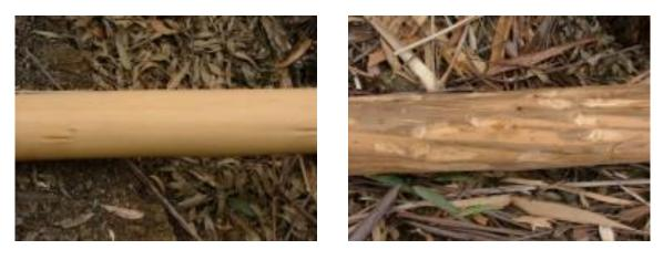
Photo 1 (left) Clean debarked log and Photo 2 (right) chiselled log<sup>3</sup>
