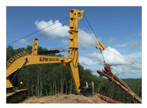
Photo 5: High power double drum shovel yarder with extended tower.9
