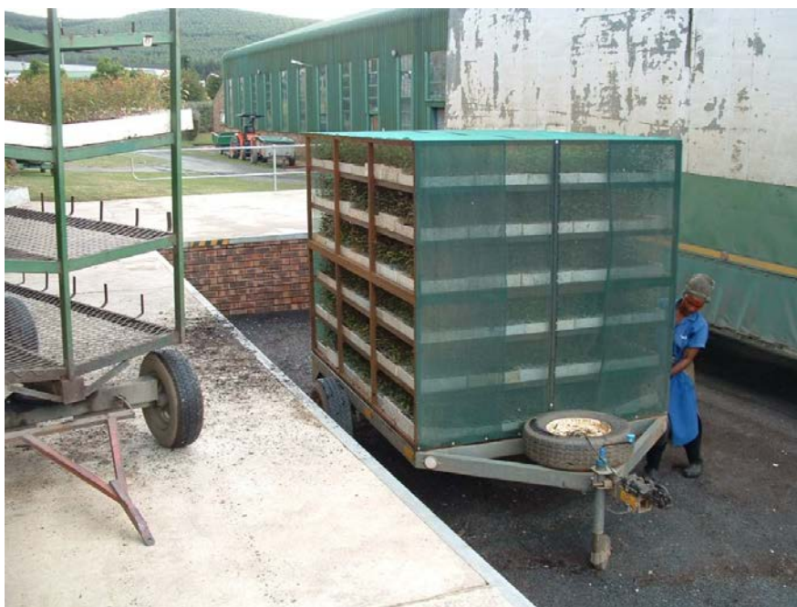
Photo 1: Seedling trailer capable of transporting \pm 10,000 seedlings in Sappi 49 trays. 1
