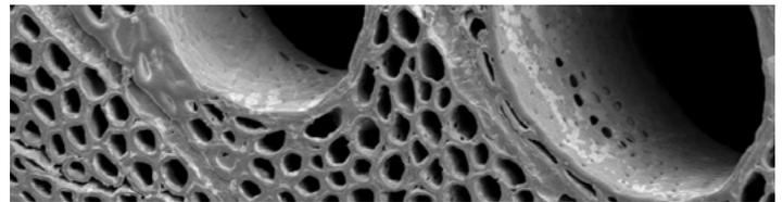
Electron microscope image of *Eucalyptus nitens*; showing wood structure.
